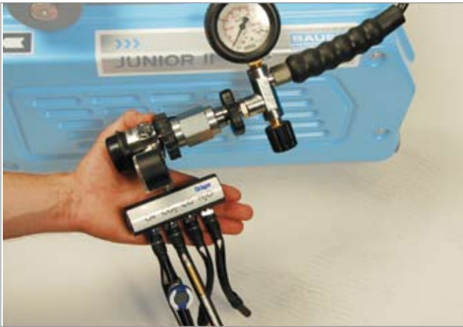
Measuring the air quality at the compressor
