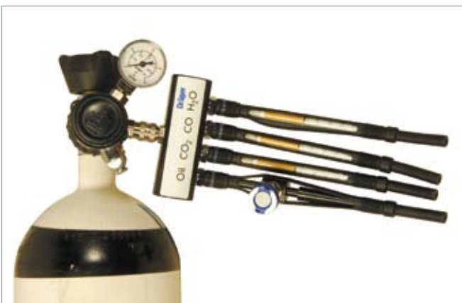
Measuring the air quality directly at the breathing air cylinder
